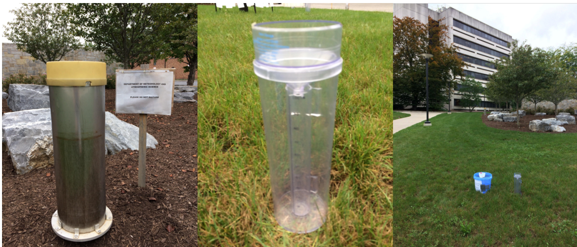
FIG. 2. Photos of the Weather Center gauge (left), commercial gauge (center), and grass lawn with all three gauges in sight (right). Some of the major obstructions are shown—including Walker Building, a stone wall, and several trees.
